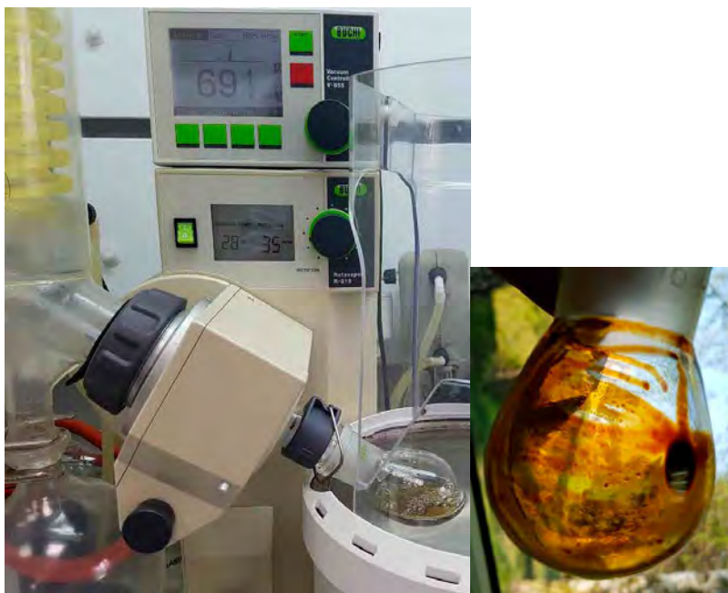
Figure 25: Rotary evaporator (left) and fats and oils extracted from WAS sample C (right)
