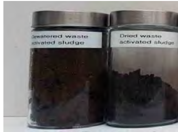
Figure 31: WAS sample A; from left to right; mechanically dewatered WAS, dried WAS sample
