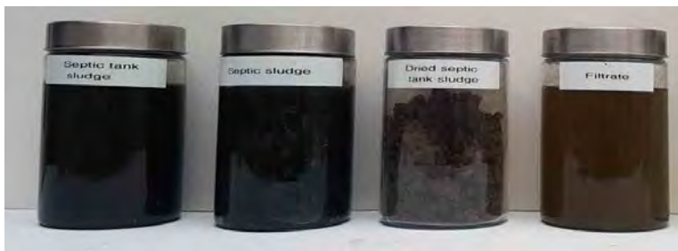
Figure 32: SS sample D; from left to right; raw SS, dewatered SS, MW dried SS sample, SS filtrate.
