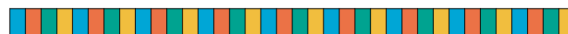
Figure 7.3: A coalesced memory layout, where each color represents the components of a single deformation gradient tensor stored. When fetching global memory utilizing the coalesced memory layout, the values of the memory addresses that the threads of a warp visit are contiguous. Consequently, the time to retrieve values from global memory is reduced.
