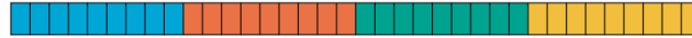
Figure 7.1: A strided memory layout, where each color represents the components of a single deformation gradient tensor stored. Aligned with the SIMT principle, each thread concurrently performs the same task. Therefore, if each thread is assigned to a single quadrature point, all threads will first load the first component of their respective deformation gradient tensor. In the strided memory layout, deformation gradient tensors are ordered one after another. Consequently, eight memory addresses are present between the values that the threads of a warp fetch.
