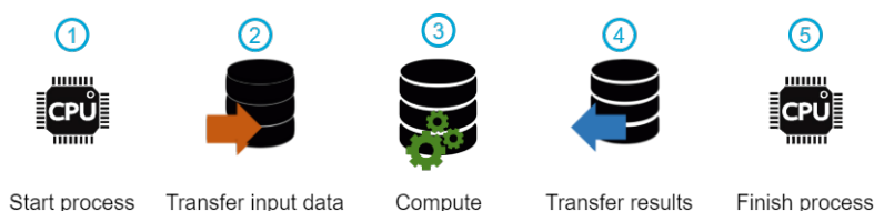
Figure 2.1: The main events present in the GPU computing process. A GPU relies on code initialization on the CPU, followed by transferring input data towards the GPU. Utilizing the input data, the GPU performs the computation and subsequently transfers the results back to the CPU. Finally, the CPU continues with its tasks and finishes the process.
