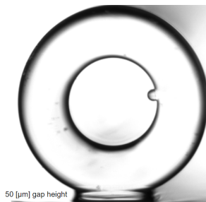
Figure 3.14: Front view of bond geometry 50 [ \mu\text{m} ] gap height.
