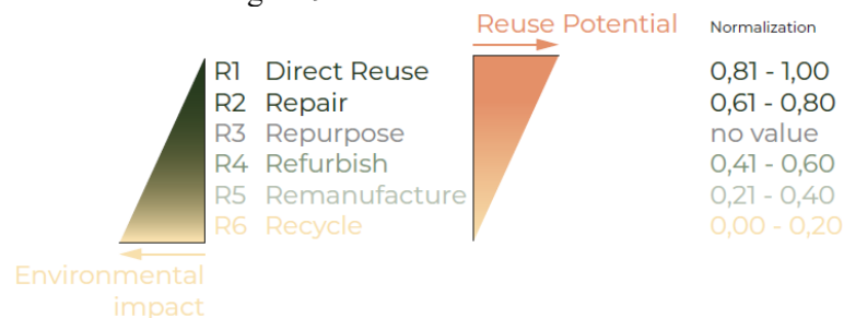
Figure 9 correlations reuse potential and environmental impact with normalization factor (made by author)
