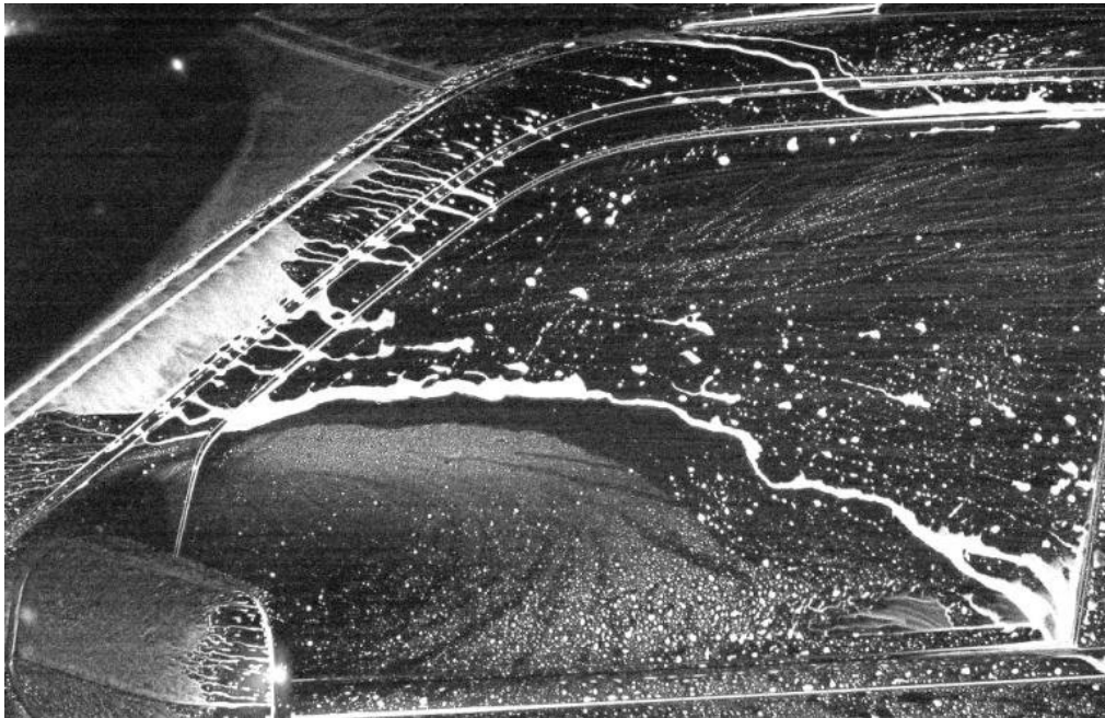
Figure 2.4: A-pillar Overflow visualized [36]
