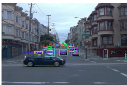
(a) A front camera image with object annotations from the Waymo [60] dataset.
