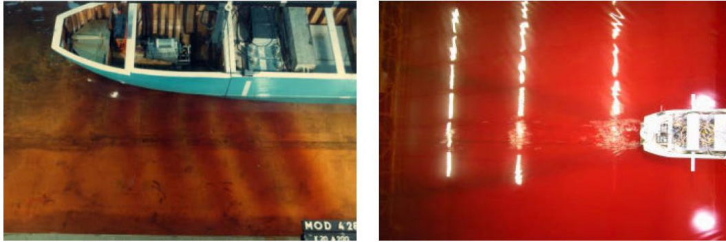
Figure 3: Propagation pattern of internal waves of the water-dense fluid interface for viscosity 0.002 Pa s (left) and 0.03 Pa s (right). The photos are taken from Delefortrie, G. & Vantorre, M. (2015).
