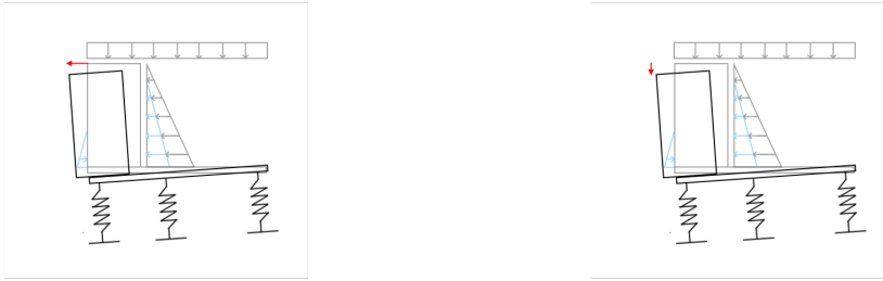
Figure 8.3: Horizontal (l) and vertical (r) displacements of the quay wall in cross-sectional direction
