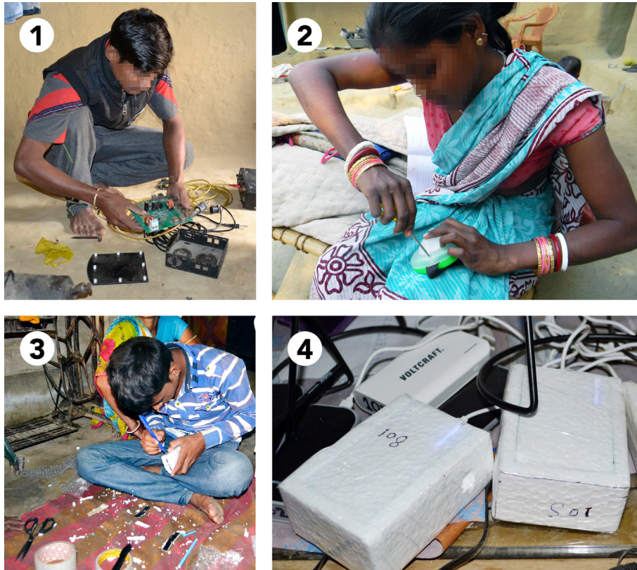
Figure 6 Re-configuration of various elements of the prototype. Please note the labels. '1': soldering of a broken energy-router; '2': energy-giver repairing a solar-lantern at Manpur; '3': a family member of energy-giver at Rampur redesigning the casing of power banks using locally available materials; and '4': redesigned cases of power banks Rampur
