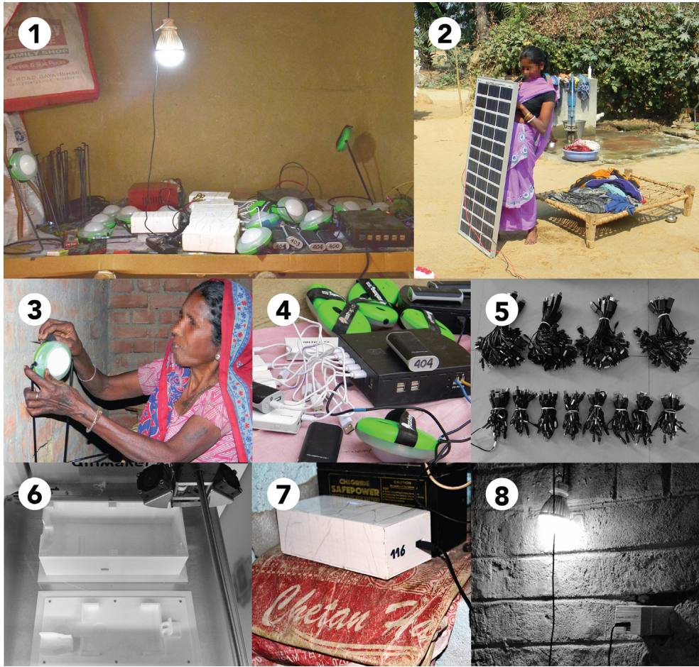
Figure 4 Off-Grid Energy Distribution Infrastructure. Note the labels: '1': charging station; '2': solar panel; '3': solar lantern; '4': energy router; '5': cables; '6': 3D printed casing of the power banks; '7': a power bank in use; '8': a LED bulb connected with a power bank
