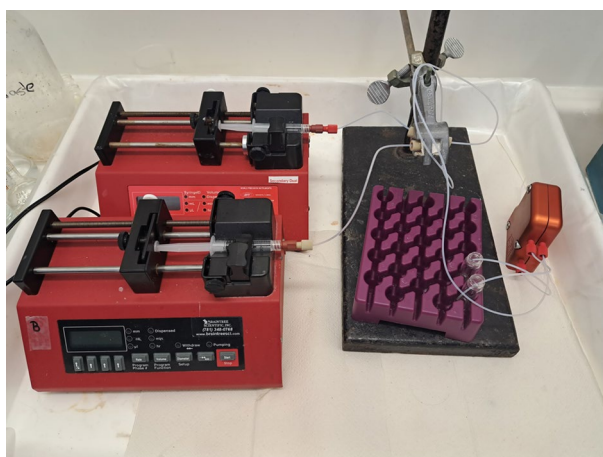
Fig. 1 Microfluidic solvent extraction set-up using a Zaiput Sep-10 membrane separator. The slug flow is created by the fluidic y-connector
