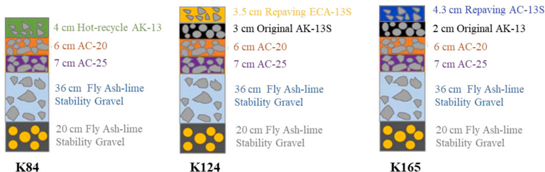
Fig. 1. The pavement structures and the maintenance history of three road sections.
