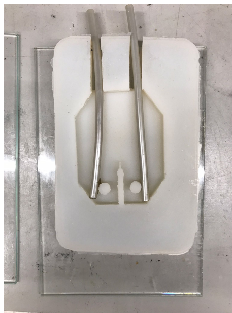
(b) Adding injection tubes
