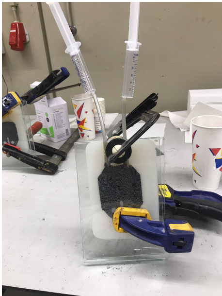
(a) Moving of injection tubes with resin level
