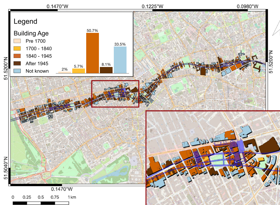
FIGURE 8 Age-based classification of the buildings between Paddington and Liverpool Street, along the Crossrail twin tunnels in central London. The Crossrail alignment is represented with a blue line
