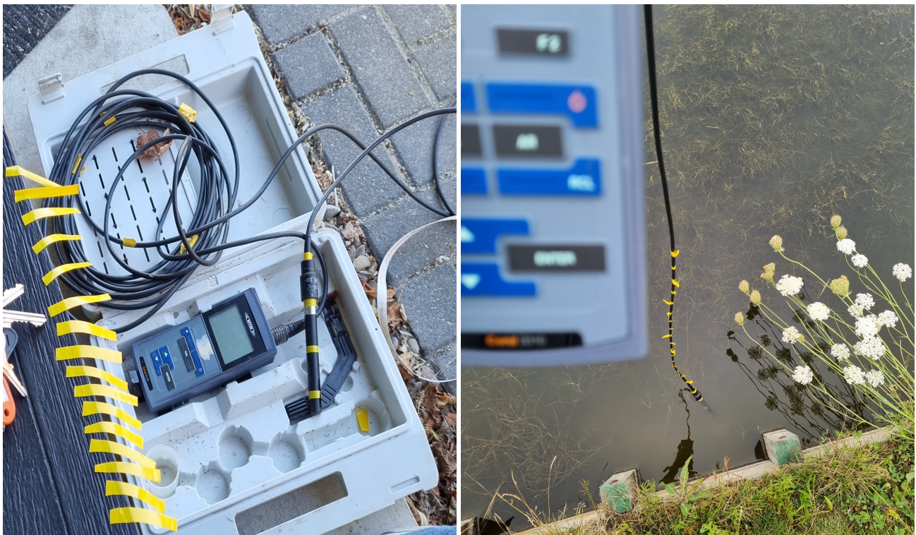
(a) Attaching the yellow tape to the cord [Own picture, 2022] (b) Measuring the conductivity over the depth using the yellow stripes [Own picture, 2022]
