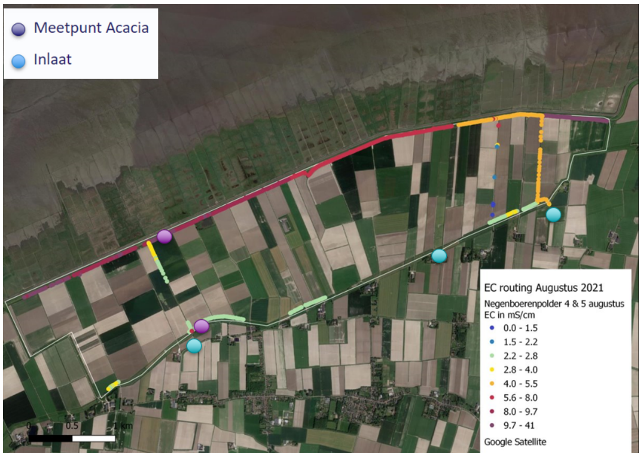
Figure 56: Routing of the Electrical Conductivity in the Negenboerenpolder during August 2021 [van der Heijden, 2021]
