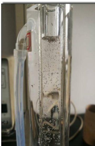
Figure 5. Apparatus setup for sand suspension ability test.
