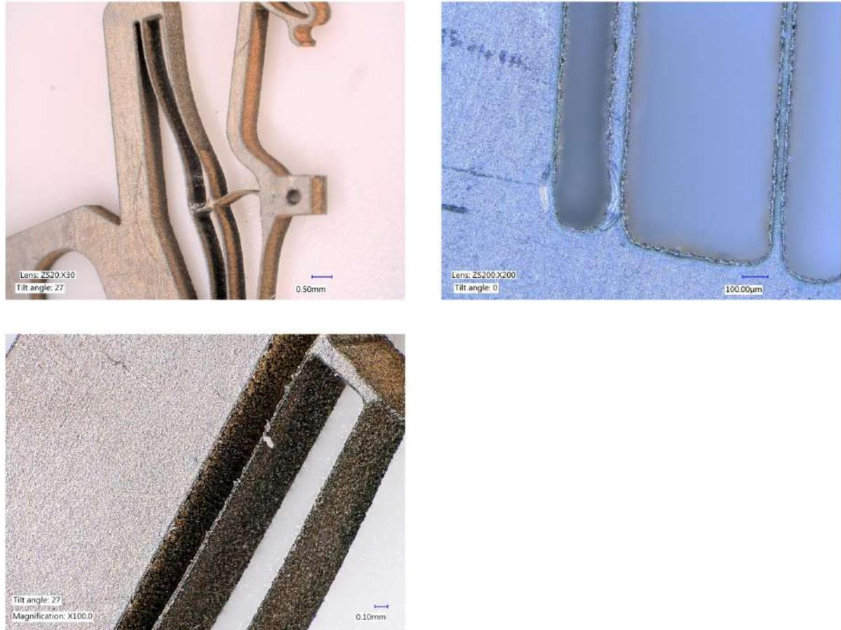
Figure C.7: Keyence microscope images of second attempt at wire EDM prototype
