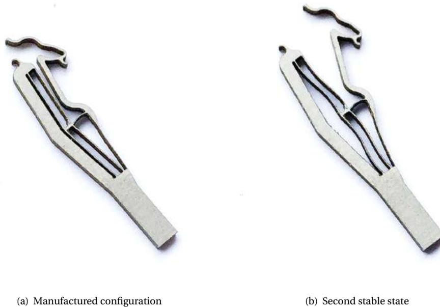
Figure C.8: Wire EDM demo prototype in two stable positions
