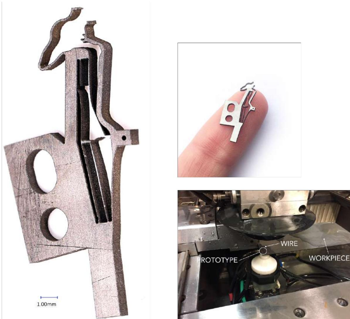
Figure C.6: Left: Keyence microscope image of first attempt at wire EDM prototype. Top right: image of first wire EDM attempt. Bottom right: Wire EDM setup during manufacture of first prototype.
