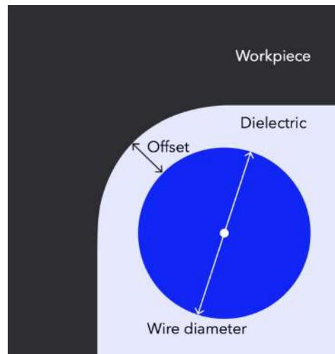
Figure C.2: Wire EDM offset
