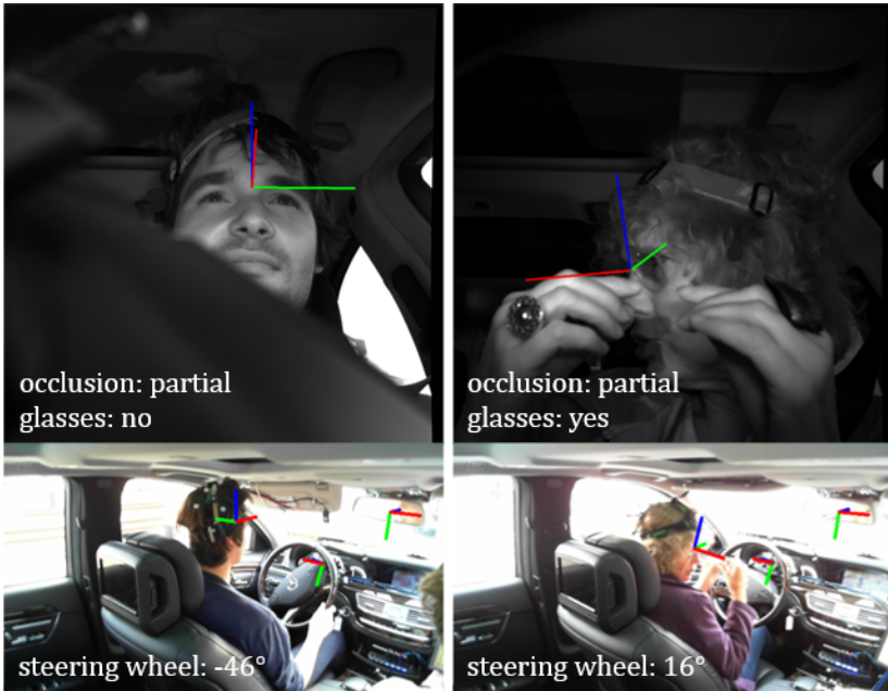
Figure 3.1: DD-Pose provides precise 6 degrees of freedom (DOF) head pose annotation for 330 k stereo image pairs acquired in an in-car environment. The benchmark offers significant out-of-plane rotations and occlusions from naturalistic behavior introduced by complex driving scenarios. Annotations for partial and full occlusions are available for each high-resolution driver camera image. An additional camera capturing the interior of the car allows for further multi-sensor driver analysis tasks.
