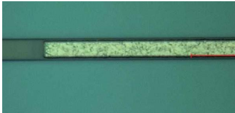
Figure 5.15. Drift of 200 nm thickness samples after 20 hours at 300 °C, (a) the full covered Al stripe. (b) the bare Al stripe.
