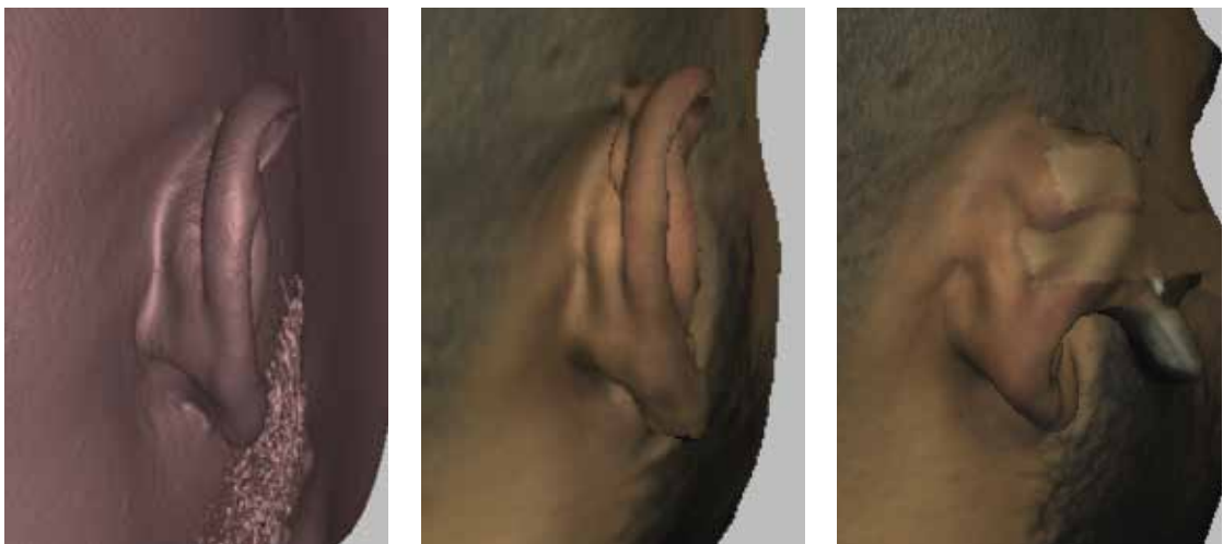
IMAGE 4a.9 Comparison between right ear scans. From left to right: Artec Spider, Artec Eva and Artec Eva with tape
