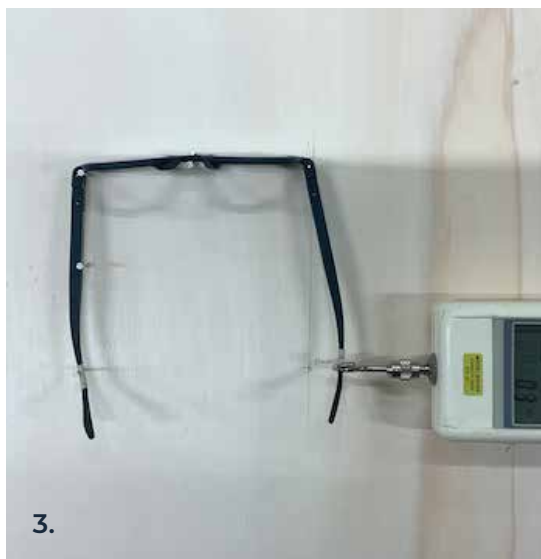
IMAGE 3b.3 Measurements in the lab to define spring force:
