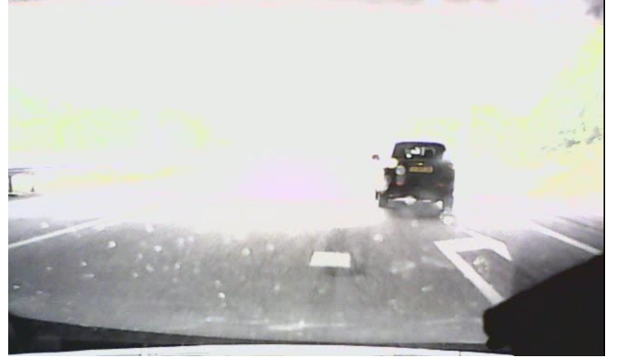
Fig. 4: The ego vehicle passes a flyover during daytime while performing a lane change. This causes glare such that the distance to the lane lines are not available.
