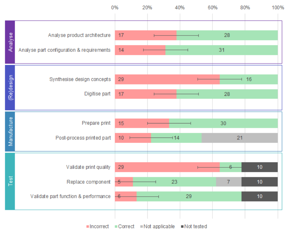
Figure 4. 3DPfR process steps (per phase) that were performed incorrectly, performed correctly, or not applicable for a particular repair case.
