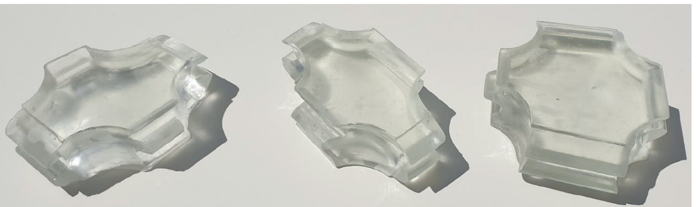
Figure 5.9: Interlocking system for a shell structure. Retrieved from Weijst (2019).
