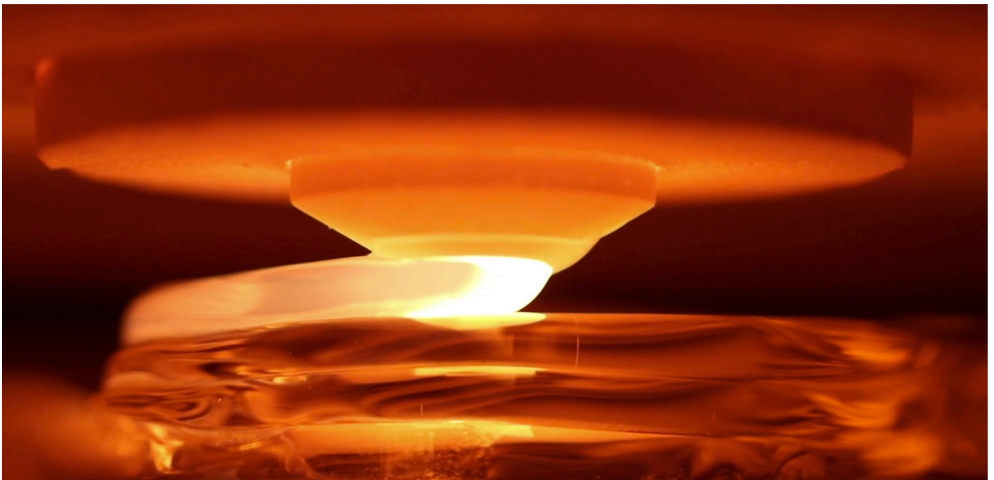
Figure 4.7: Glass 3D printing process (top) and result glass 3D print (left). Retrieved from Drupa (2015).
