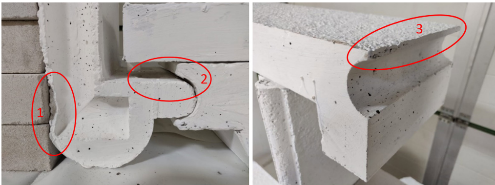
Figure 8.7: Errors in the prototypes. 1) Damage in the edges of the interlocking when removing the mould, 2) Miscalculation when building the mould, 3) Too thin edge for web interlocking.
