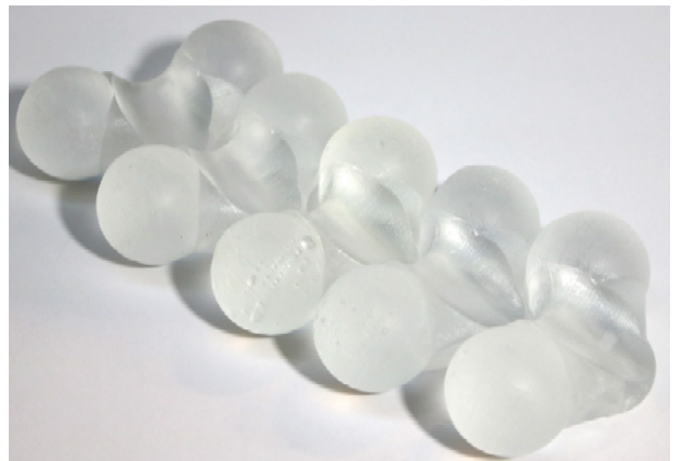
Figure 5.7: Dry-assembly interlocking glass bridge structure. Retrieved from Aurik, Snijder, Noteboom, Nijse, & Louter (2018).
