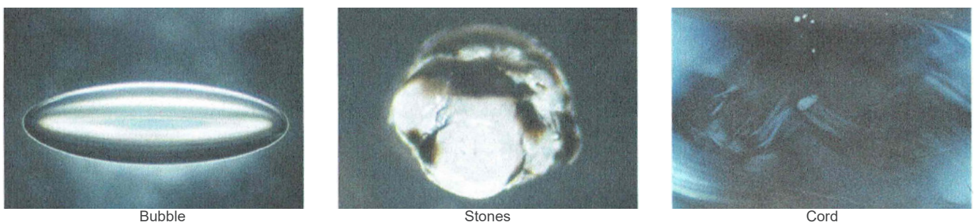
Figure 4.12: Flaws in cast glass. Retrieved from Oikonomopoulou (2019).
