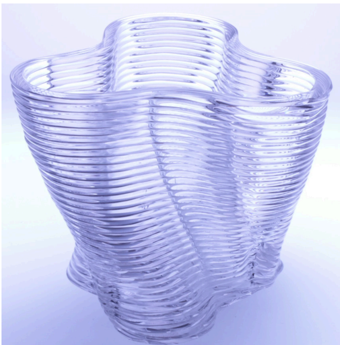
Figure 4.7: Glass 3D printing process (top) and result glass 3D print (left). Retrieved from Drupa (2015).
