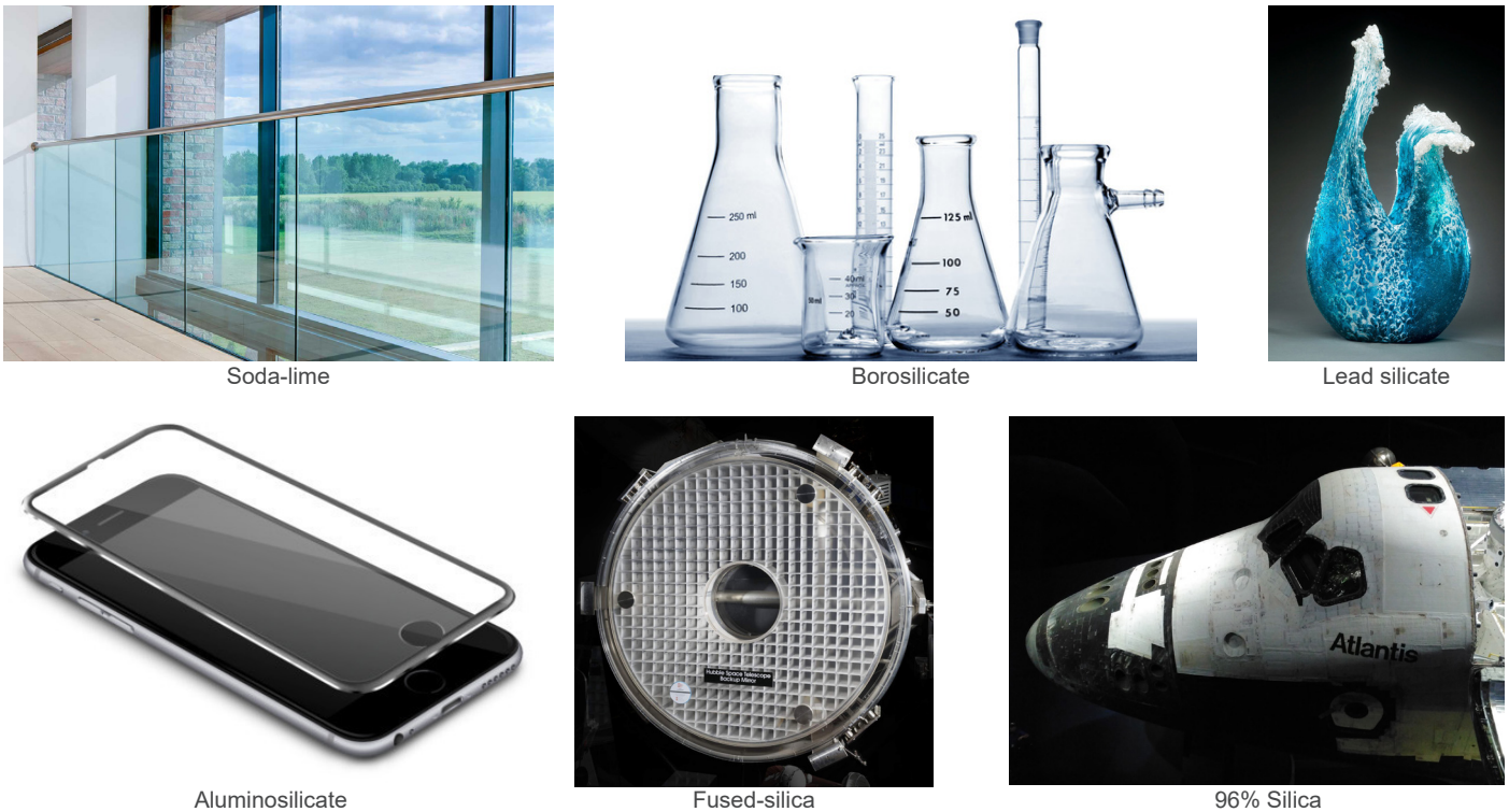
Figure 4.2: Application of glass types. Retrieved from Jackofglass (n.d.), Smithsonian (2019), Yang (2015), Corning (n.d.), Heraldssystem (2019) and Spacemood (n.d.).
