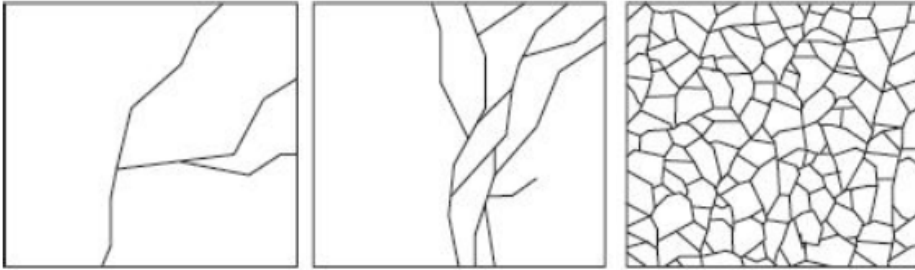
Figure 4.3b: Failure pattern of strengthened float glass: annealed (left), heat strengthened (middle) and tempered (right). Retrieved from Louter (2011).
