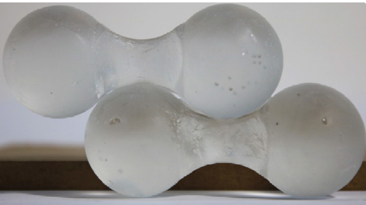
Figure 5.8: Interlocking system for a dome structure. Retrieved from Janssens (2018).
