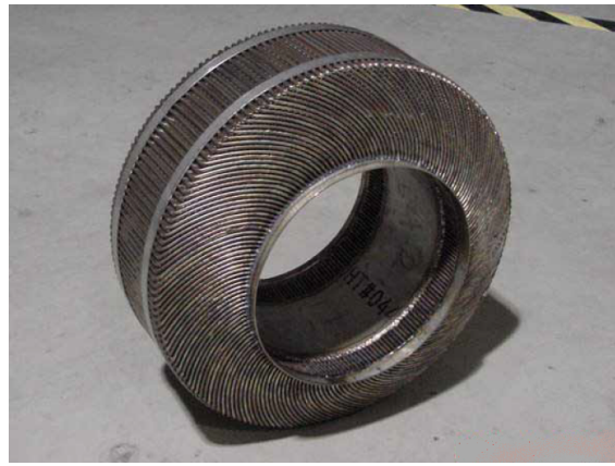
Figure 2.7: Capstone complete assembly for 200 kW microturbine [8]
