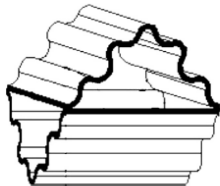
Figure 2.26: Cross corrugated surface with additional corrugations [3]
