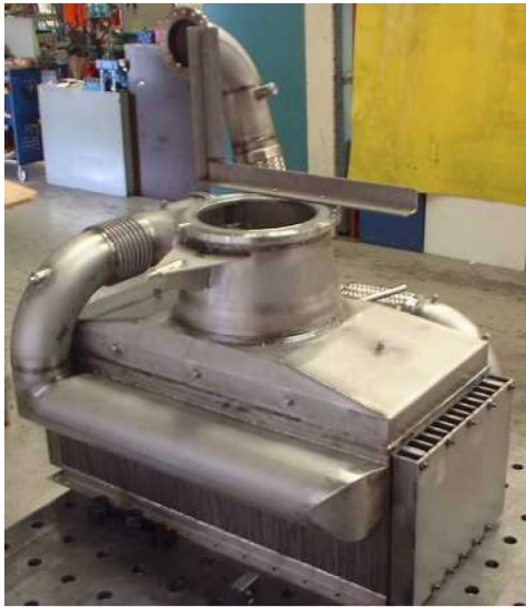
Figure 2.11: RSAB prototype for 100kW microturbine [11]
