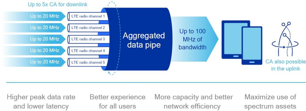
Figure 2.2: Carrier Aggregation in LTE [33]
