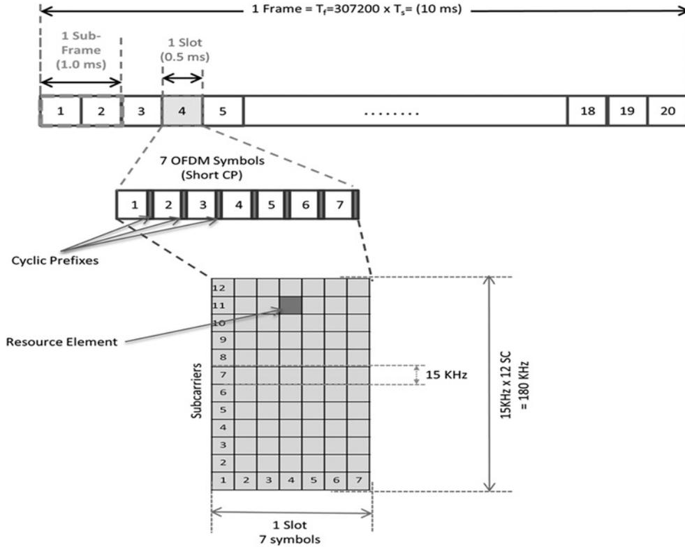
Figure 2.1: Radio resource structure in FDD mode: 4G LTE and one configuration option for 5G NR
