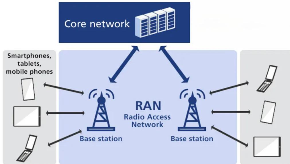
Figure 1.2: Simplified diagram of a cellular network.
