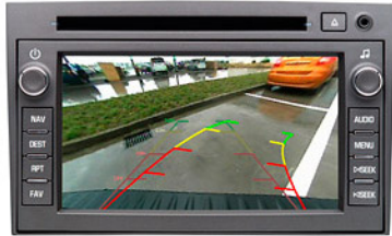
Figure 2: The Delphi Parking Guidance System superimposes guidelines on the vehicle display, courtesy of Delphi Automotive LLP
