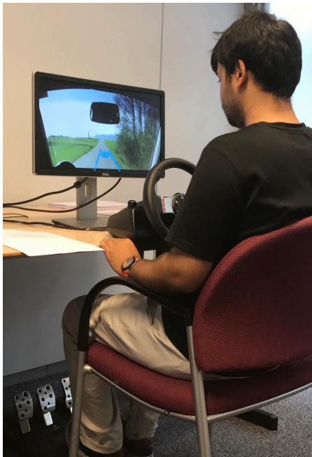
Figure 3: Non-interactive driving simulation setup with real-world driving videos
