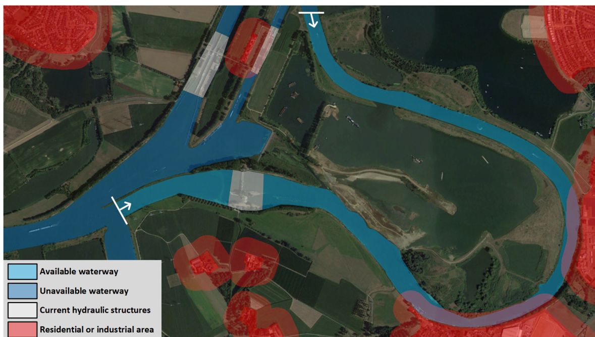
Figure 5.2: Sieve analysis of the possible locations to construct the new weir at Linne (Beeldmateriaal Nederland, 2023)
