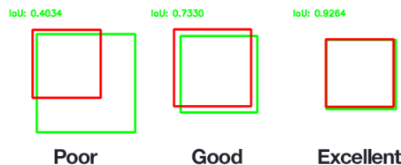
Fig. 8: Example IoU scores for bounding box evaluation. Taken from Wikipedia [30].
