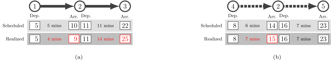
Fig. D.9. An illustration of the optimized schedule versus the realized schedule for a bus on routes r_1 and r_2 respectively.
