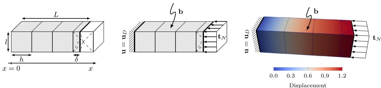
**Fig. 8** Single material linear elastic bar with varying sliver size and ghost penalty parameter: problem setup, boundary conditions and solution for quadratic displacement solution using quadratic B-splines
