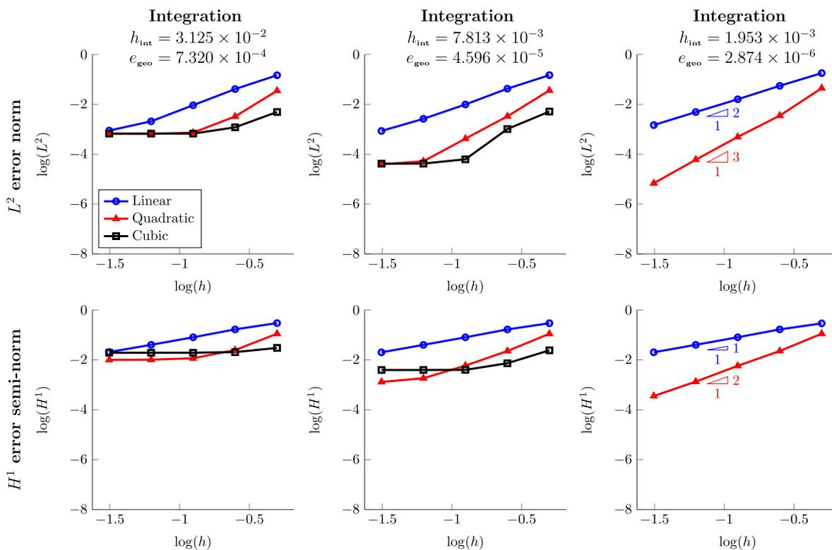
**Fig. 21** Heated spherical inclusion in an infinite medium, refinement of the temperature field for three different fixed geometry refinements  $h_{\text{int}} = 3.125e^{-2}$ ,  $7.813e^{-3}$ , and  $1.953e^{-3}$  m
