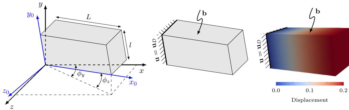
**Fig. 13** An immersed single elastic material bar rotated in a fixed 3D background mesh: problem setup, boundary conditions and solution using quadratic B-spline with rotation angles  $\phi_y = 20^\circ$ ,  $\phi_z = 20^\circ$  and a mesh size  $h = 0.125$  m
