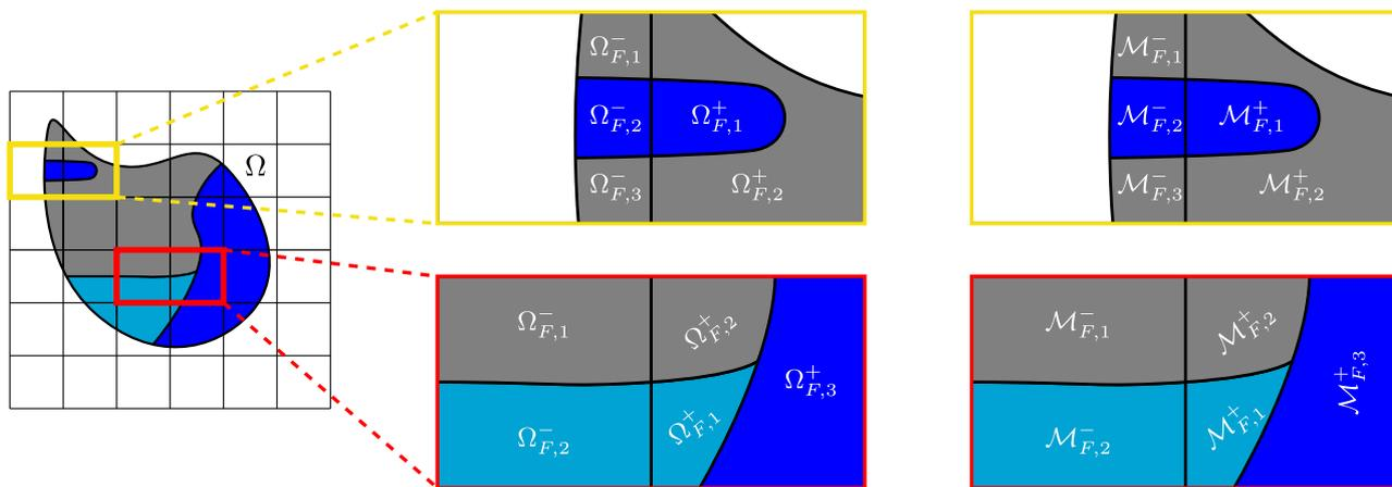
**Fig. 6** Subdivision of  $\Omega_F^+$  and  $\Omega_F^-$  into connected subdomains  $\Omega_{F,i}^+$ ,  $i = 1, \dots, N_F^+$  and  $\Omega_{F,j}^-$ ,  $j = 1, \dots, N_F^-$  for the face-oriented ghost stabilization for a three-material problem
