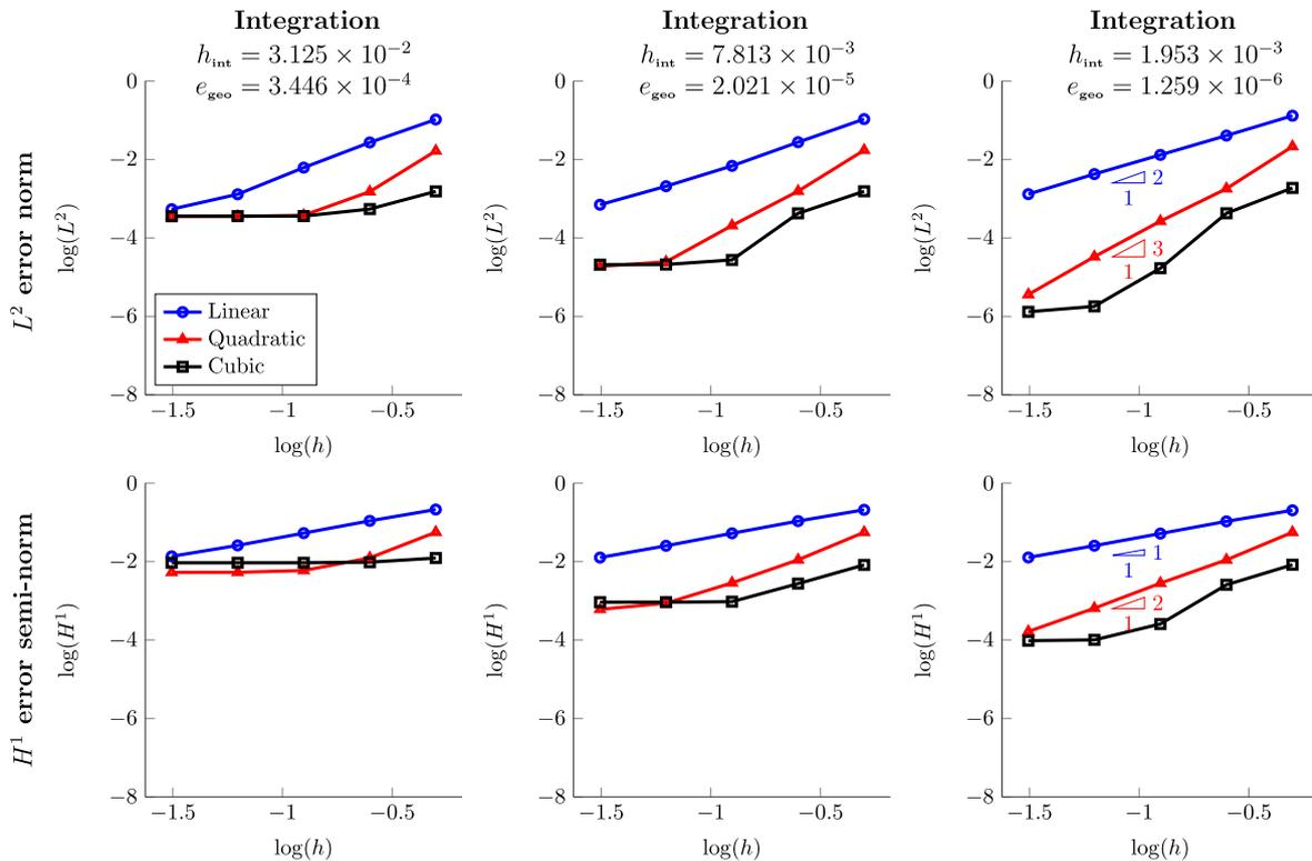
**Fig. 20** Heated cylindrical inclusion in an infinite medium, refinement of the temperature field for three different fixed geometry refinements  $h_{\text{int}} = 3.125e^{-2}$ ,  $7.813e^{-3}$ , and  $1.953e^{-3}$  m
