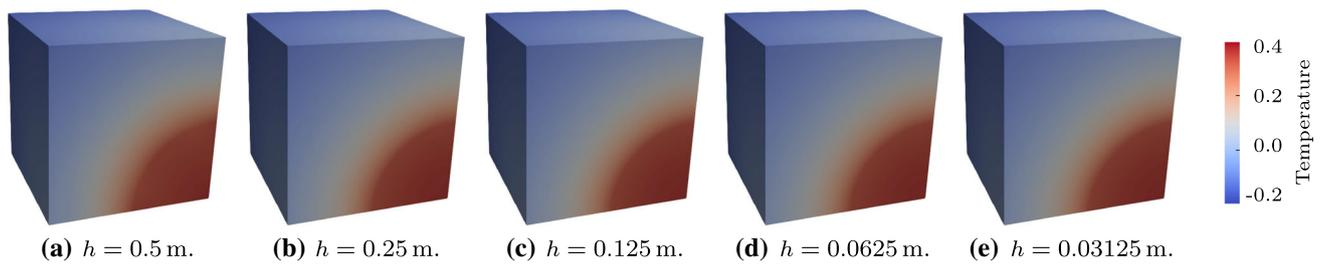
**Fig. 19** Heated inclusion in an infinite medium, refinement of the temperature field with a fixed geometry field  $h_{\text{int}} = 0.03125$  m, solution using quadratic B-splines in three dimensions
