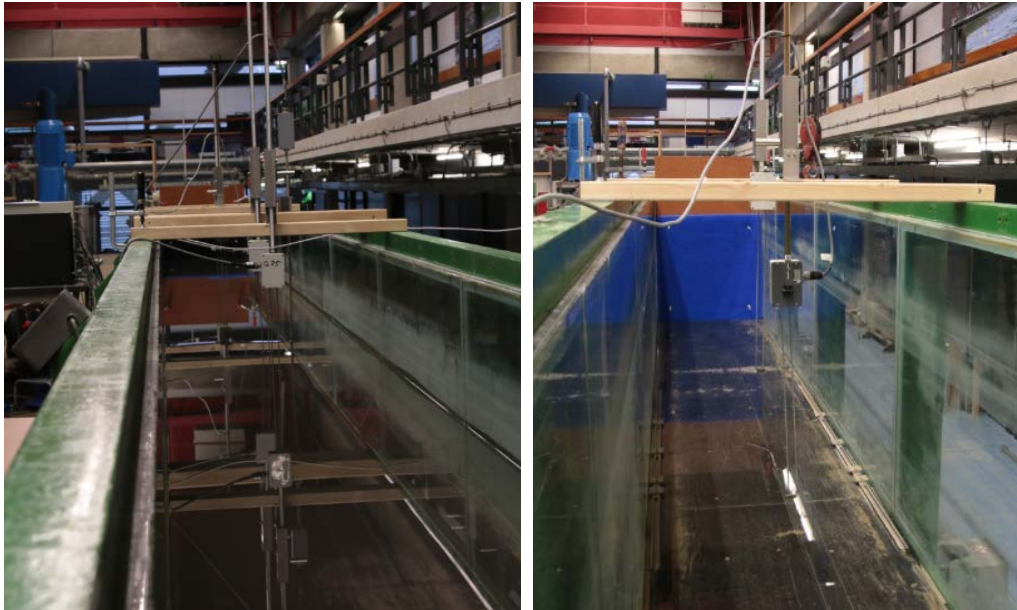
Figure 93: Gauges set-up in the flume
