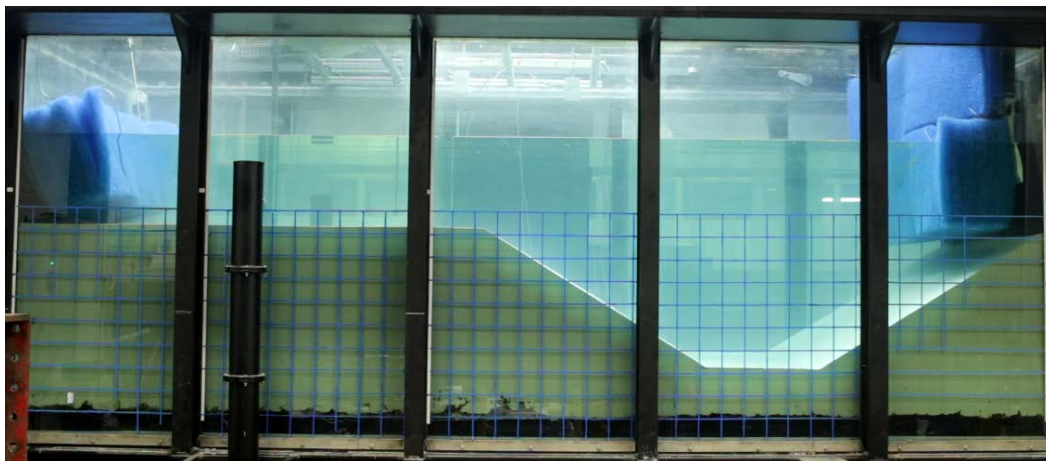
Figure 100: Wave absorber installed inside the static liquefaction tank.
