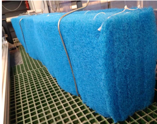
Figure 99: Final design of a wave absorbing element: 6 layers of Japanese filter with total thickness of 30 cm.
