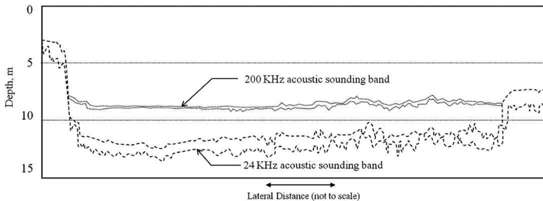
**Figure 2: Dual-frequency echo sounding in a channel with fluid mud layers.**
