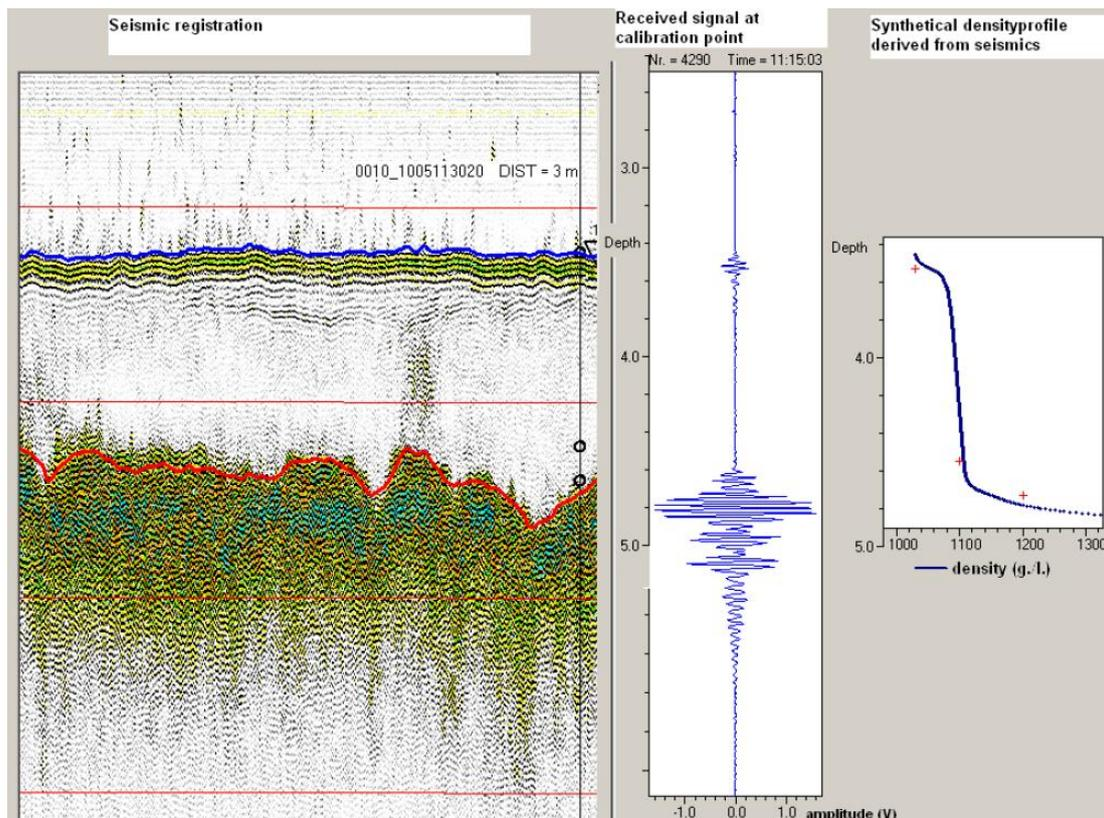
**Figure 3: The density 'calibration' to the measured acoustic signal using SILAS
