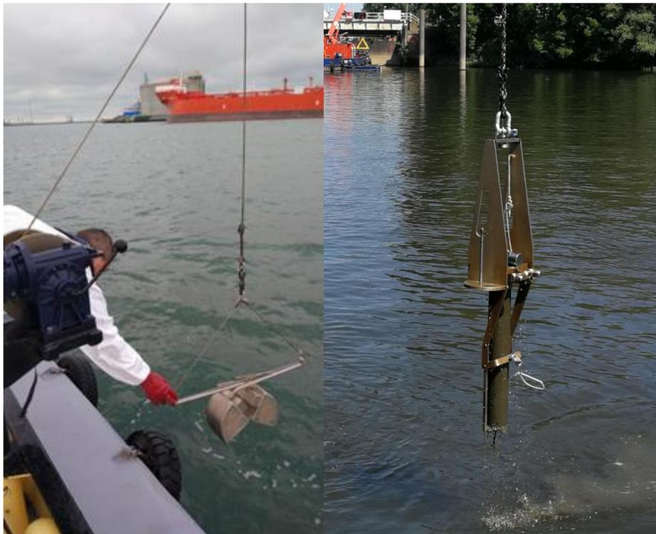
**Figure 7: Disturbed (left) and undisturbed (right) sampling methods**
