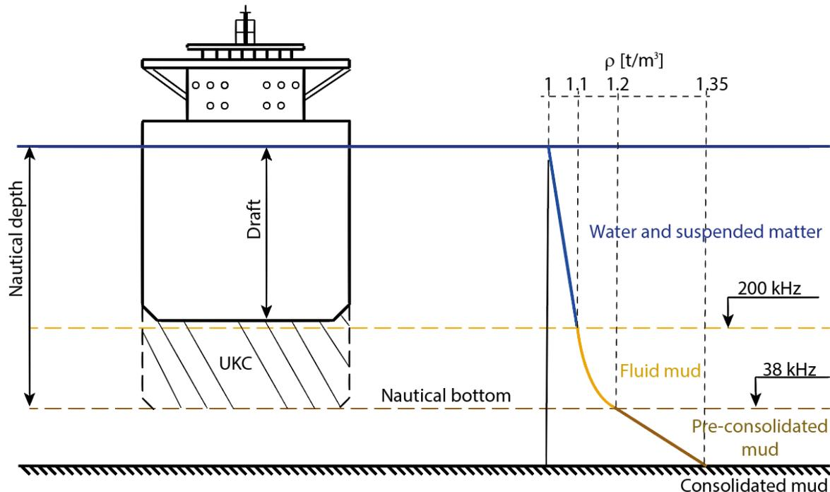
**Figure 1. The nautical bottom concept at the Port of Rotterdam for the density limit of 1.2 t/m<sup>3</sup>. From Kirichek et. al., 2018.**
