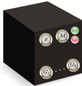
Figure 4.2: Gate set tomography treats the studied quantum processor as a black box. Circuits can be run by pressing the processor's buttons, but how the buttons look exactly (in the mathematical sense) is unknown. Figure taken from Blume-Kohout et al [27].
