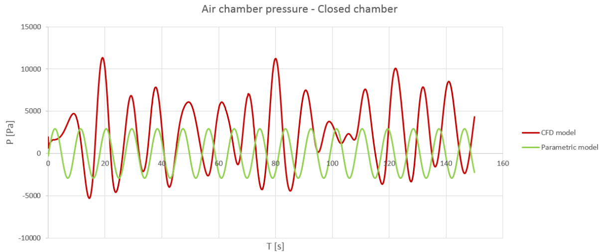
Figure 50 - Air chamber pressure of both models ( A_{inc} = 0.5 \text{ m} , T = 9 \text{ s} , closed chamber)
