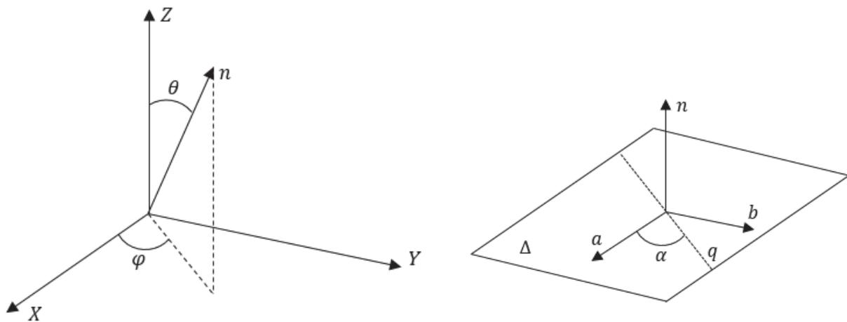
Figure 5: Determination of the orientation of the normal to the critical plane using the angles  $\varphi$  and  $\theta$  (a) Determination of the orientation of the local coordinate system of the critical plane  $abn$  using angle  $\alpha$ ; (b) Reproduced from [35].
