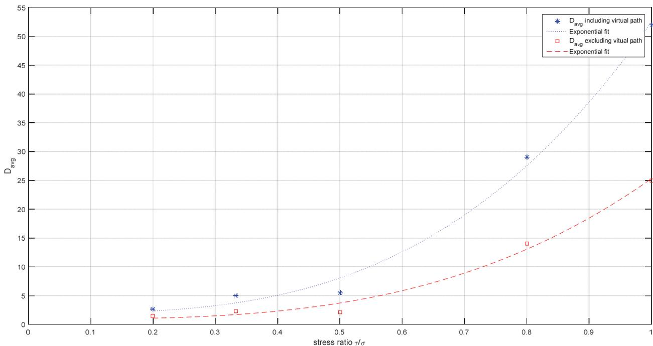
Figure 12: Graph showing the exponential increase of fatigue damage with increasing stress amplitude ratio considering PDMR based cycle counting
