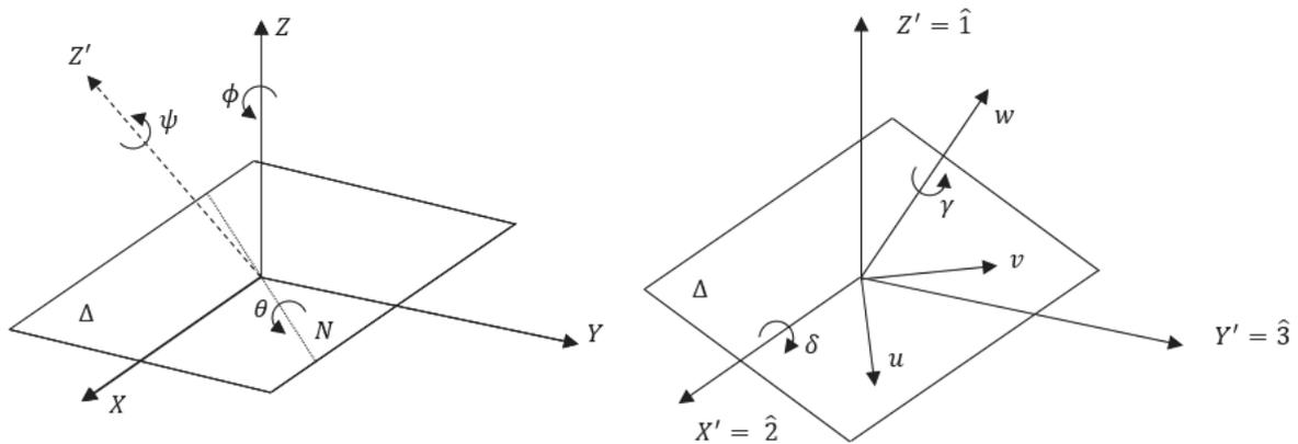
Figure 3: Representation of the counter clockwise rotations about the  $Z, N$  and  $Z'$  axis, defined through three Euler angles  $\theta, \psi, \phi$  (a) Relationship between the two spherical angles  $\delta$  and  $\gamma$  with respect to the local coordinate system with axes  $uvw$  (b); Reproduced from [32].
