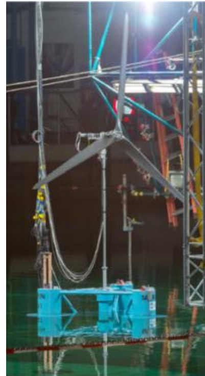
Figure 7: An image of the tested FOWT in the MARIN basin, note the large data cable bundle, taken from (Robertson, 2017)
