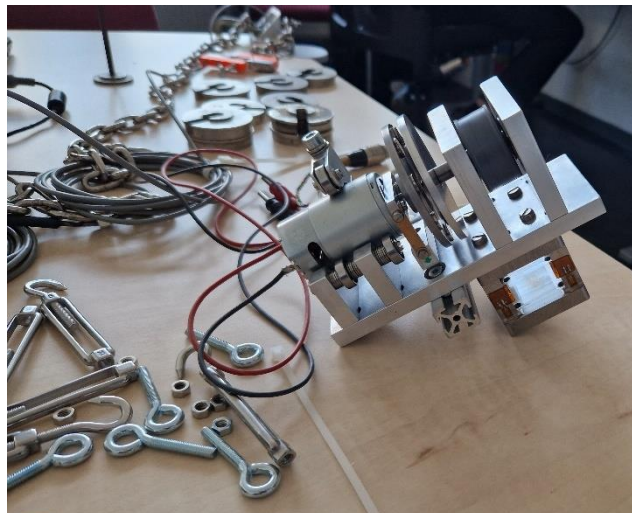
Figure 21: Photo of the wind device, clearly showing the two disks, these were later covered up for safety. The winch is visible on the right. The background shows some of the weights used for calibration.
