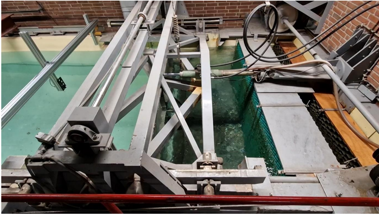
Figure 16: Wave maker of towing tank number 2 in piston configuration
