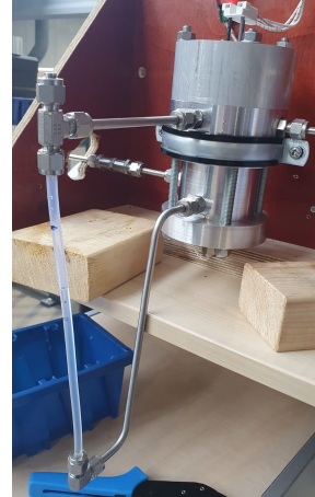
Figure 3.4: Loop outside of compressor casing to let both the top and bottom chamber equalize in pressure without enabling oil to flow between both chambers.
