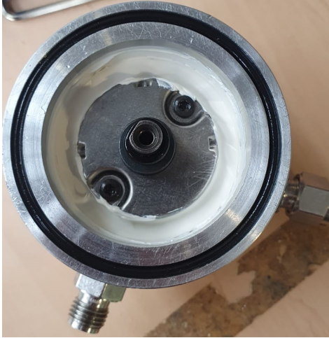
Figure 3.3: Sealing applied to inside of the compressor casing to prevent flow back into oil reservoir.
