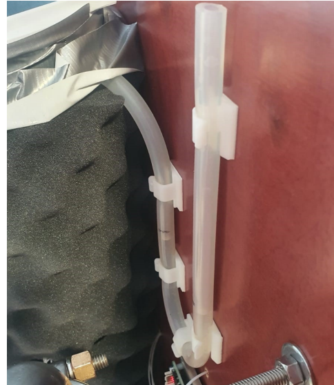
Figure 3.9: Water seal in place to estimate pressure drop over the cooling fan.
