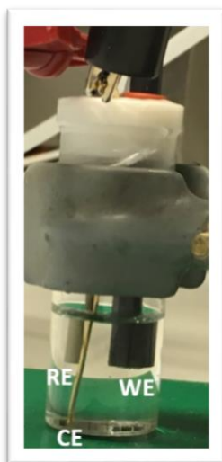
Figure 3-3. Picture of the electrochemical cell, showing RE, WE, CE.
