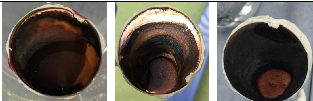
Figure A- 6. Pictures of the copper electrode surface after growing nanostructures for 30 m (left), 3 h (middle) and 24 h (right).
