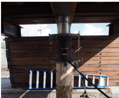
(a) Load-cell and LVDT's on pile head
