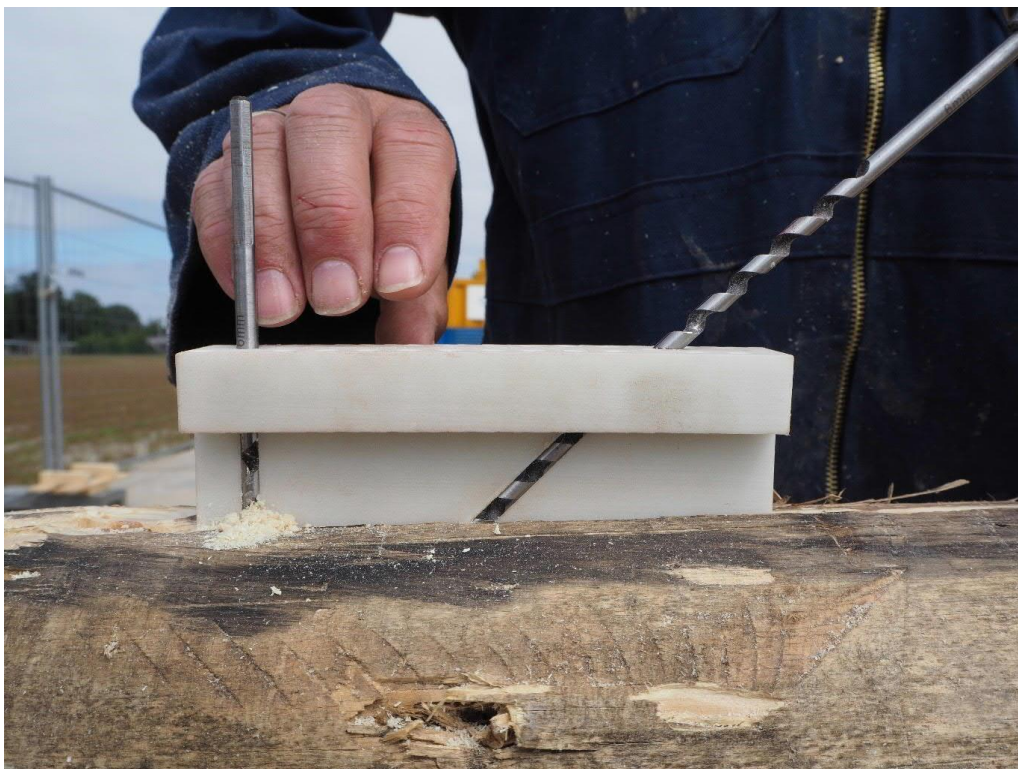
Figure E.4: Preparation: Drilling at tip for fiber loop
