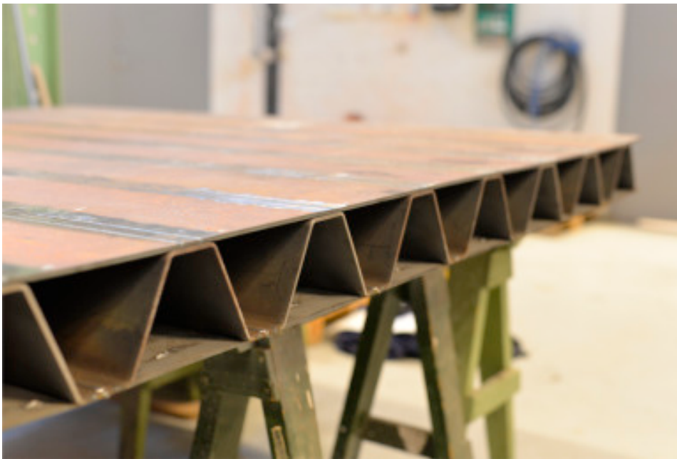
Figure 1.3: Corrugated Core Sandwich Steel Panel, Nilsson et al. [25]
