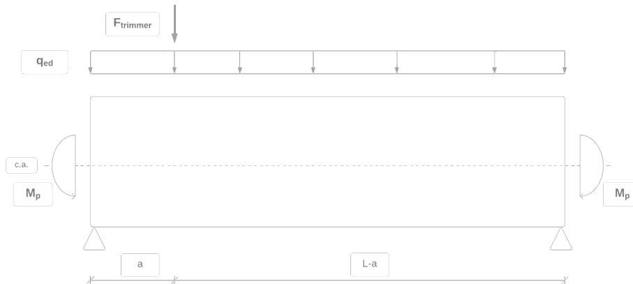
Figure 8.8: Loading scheme with an additional trimmer beam
