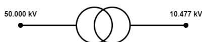
Figure 4.4: Depiction of the voltage drop over the transformer connecting the HV grid to the MV grid in PowerFactory. The rated voltage for the MV grid is 10.5 kV, however the transformer imposes a drop to 10.477 kV.
