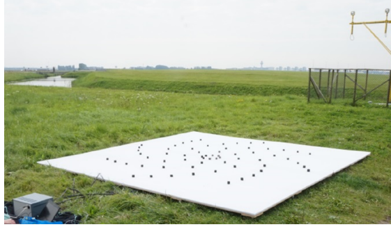
Fig. 2 Acoustic camera used to record the flyovers at Schiphol Airport.
