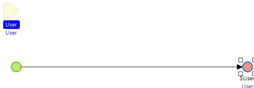
Figure 2.3: An empty Microflow consisting of a Start and End Point with a User object as input parameter and return variable.
