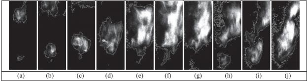
Figure 3 Sequential images show ignition kernel cluster formation and development during ignition process. Time interval between above images is 2 milliseconds.
