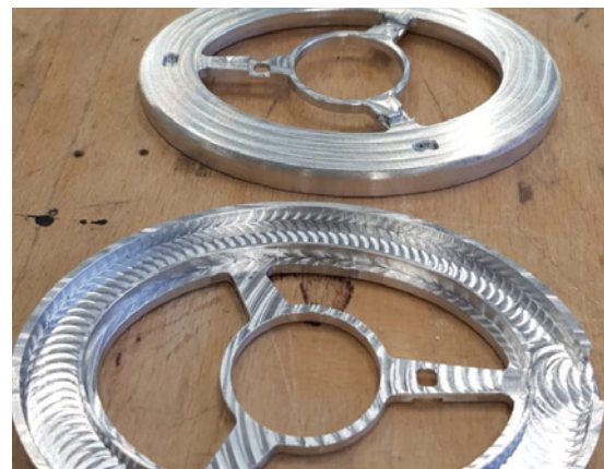
Figure 93. CNC machined aluminium earcup
