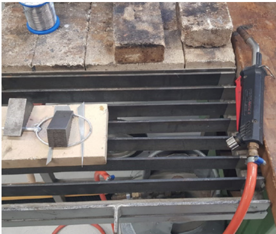
Figure 94. Brazing connection to earcup
