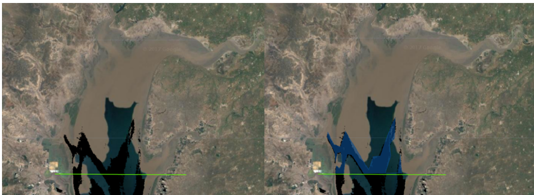
Figure G.10: Occurrence 80% (left), drawn polygon to compute this surface area (right)
