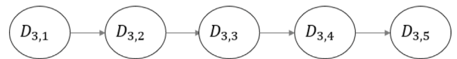
Fig. 4. T3S2 Inter-axle distances GCBN. D_{i,j} denotes a random variable representing the j th inter-axle distance of the vehicle type i ( i = 3 correspond to vehicle type T3S2). D_{i,1} is the distance between the front of the vehicle and the first axle, D_{i,2} is the distance of the first axle to the second, and so on. The arcs correspond to the (un)conditional rank correlations between individual inter-axle distances.
