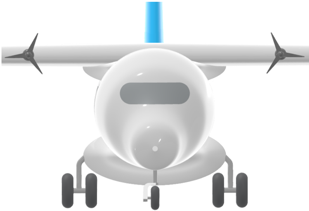
Figure 12.8: Rendered model with gear and fairing
