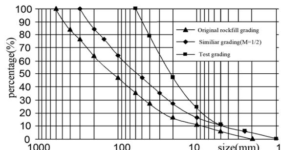
Fig. 1. Comparison of the original grading and the test grading
