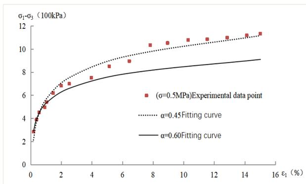
Fig.19. Comparison Fitting diagram of  $\sigma=0.5MPa$
