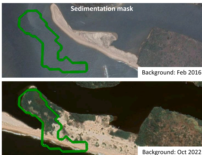
Fig. 11. Sedimentation mask (obtained by comparing the averaged image of 2020 and the one of 2017), VV polarization, represented by the green polygon. In the background maps (Google Earth) it is possible to notice the evolution of the sediments over time (top panel: before the study period; bottom panel: after the study period).
